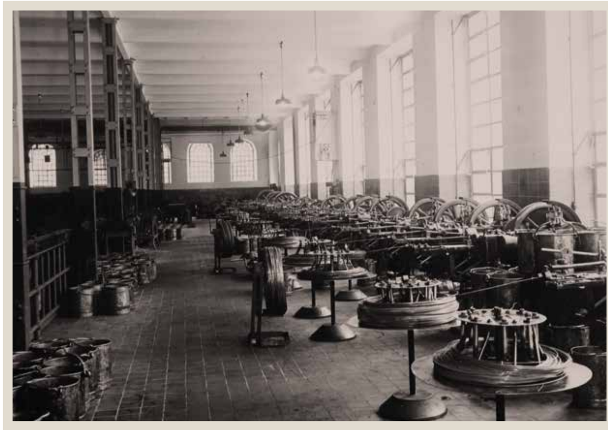
ABC press: The pressing machines are lined up along the window front, with the reels with the wire coils to the left.
