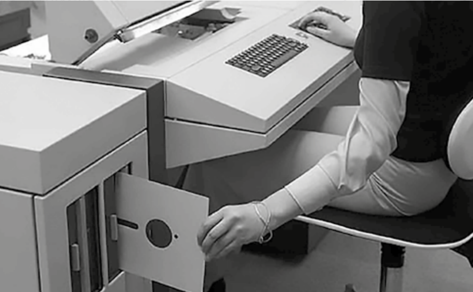
Floppy disk: Starting in 1973, a recordable and exchangeable storage medium in the form of a soft, flexible plastic disk became available for the first time.
