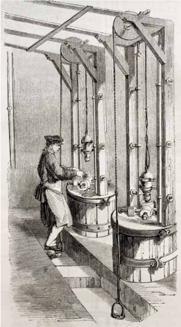
Drop hammers in a thimble and sewing needle factory
