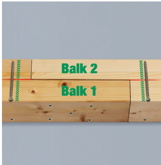
Balkverlenging met overlap (inkeping) dwarstrekkerversterking
